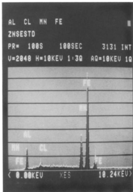
Figure 7 EDS analysis of pit formed on Fe-8.25 Al-29.95 Mn-0.85 C alloy, solution-treated.
